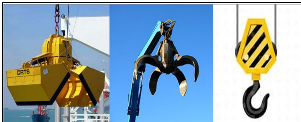
Figure-2.7 Lifting arrangements – Grab/Claw/Hook
