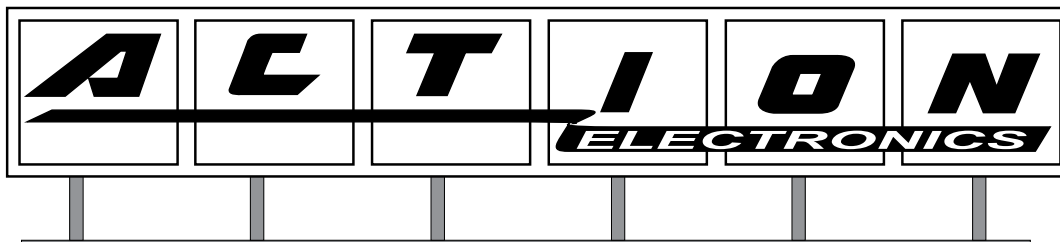
Figure 13-5: Sign area must include vertical and horizontal spacing between letters conveying the sign's message.
